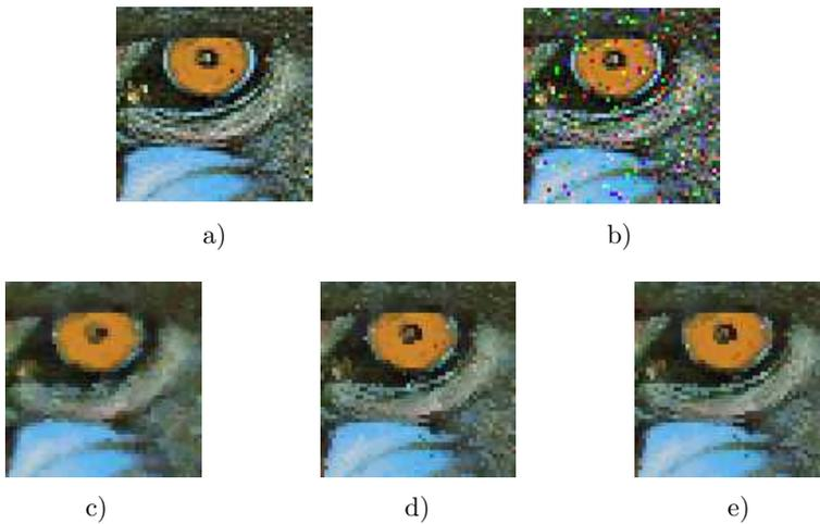
Fig. 5. Filtration results. a) original, b) noisy image, c) VMF  $3 \times 3$  window, d) floating point PGF, e) PGF customized for FPGA.
