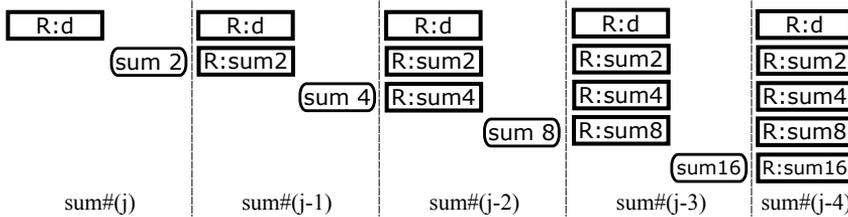
Fig. 3. Summation tree for  $a_1$  and  $a_2$  calculation.  $R$  – register,  $j$  – number of a discrete sample
