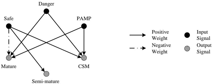
Figure 1. Abstract signal processing model in DCA
