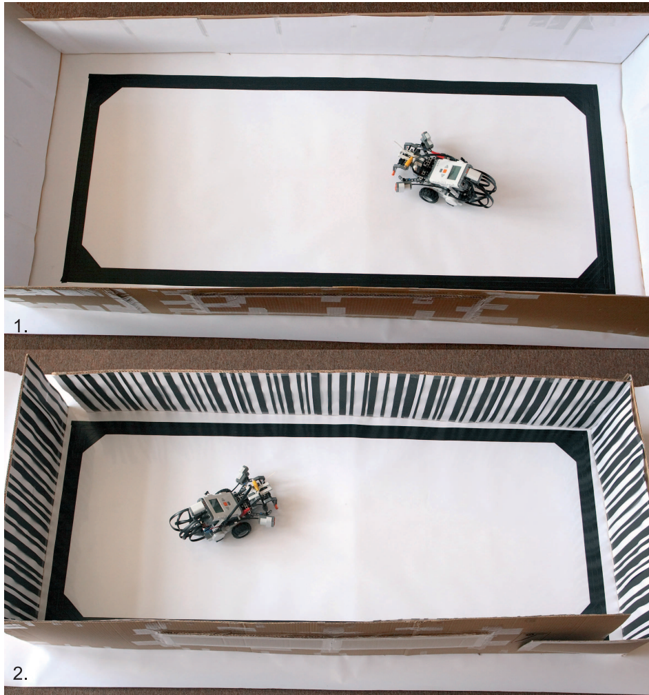
Fig. 6. Part 1) the scene with white walls; Part 2) the scene with a texture of black and white stripes
