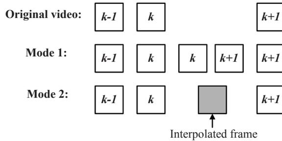
Fig. 4. The modes of joint frame duplication/interpolation
