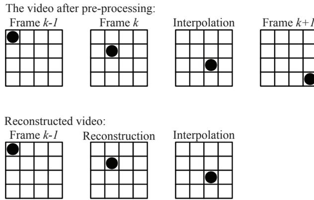
Fig. 3. MCI for frame  $k$  with pre-processing
