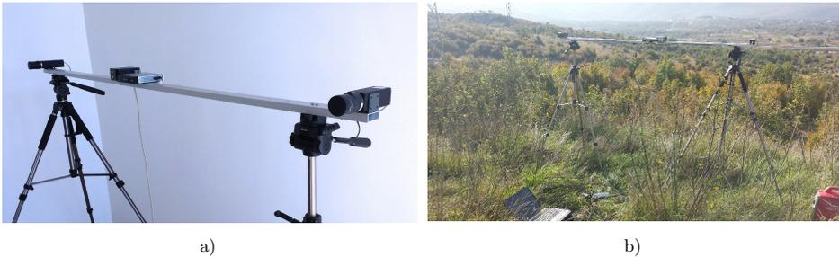
Figure 7. The stereo system used for evaluation, a) in laboratory environment, and b) in natural environment
