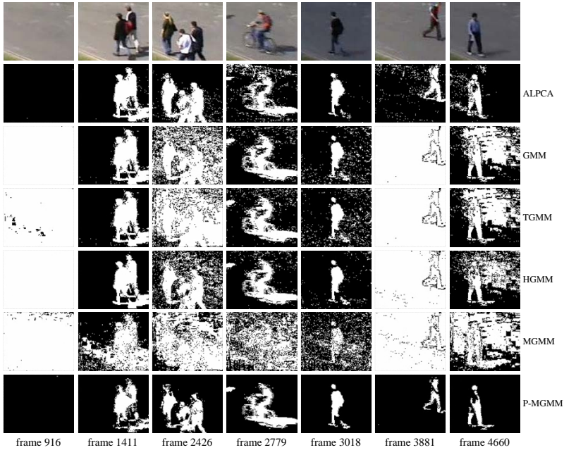
Figure 6. Experimental results on PETS01-D3-T-C1 under complex illumination variations with l = 47 , M = 102 . Each column illustrates the detection results of the chosen area at different frames in different video clips. Parameters of P-MGMM for PETS01-D3-T-C1 are given as follows: K = 3 , T = 0.34 , \sigma_{low} = 1 , \alpha = 0.005 , and S = 3 when the sub-sequence is non-stationary.
