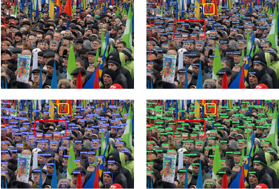
Figure 4. Inference results compared between traditional NMS (bottom left), Soft-NMS (top right) and our SF-NMS (bottom right). Our proposed SF-NMS performs better in crowded scenes.
