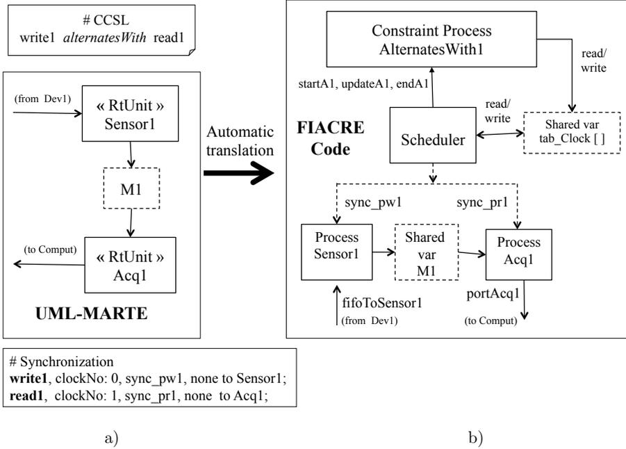
Figure 7. Illustration of a part of the generated FIACRE program
