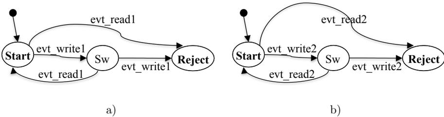
Figure 10. Observer automata corresponding to properties *P1a* and *P1b*
