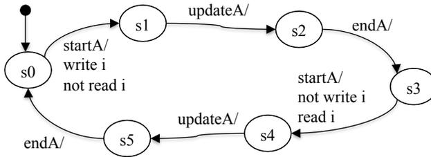
Figure 6. Automaton for the constraint  $write_i$  *alternatesWith*  $read_i$
