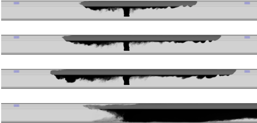
Figure 2. Smoke development in selected part of the tunnel at the 50 th , 53 th , 55 th and 137 th second of the simulation
