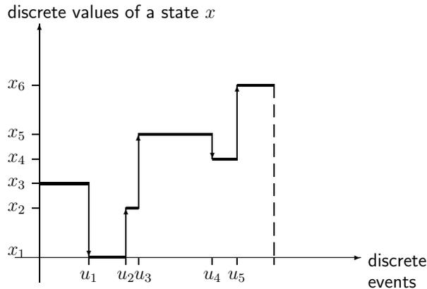
Fig. 1. The development of the state in the simple example of DEDS
