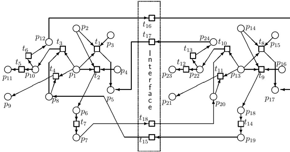
Fig. 9. The Petri net-based model of the two agents negotiation
