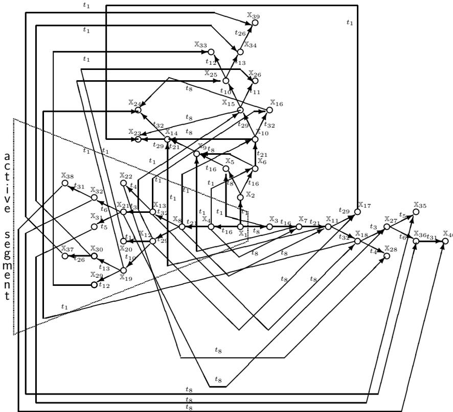
Fig. 17. The reachability graph of the three agents cooperation developed from the given initial state. The *active segment* indicates the part when  $A_1$  or  $A_2$  solves the part when  $A_3$
