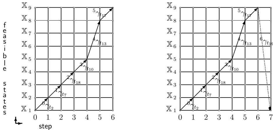
Fig. 15. The state trajectories at the cooperation of  $A_{sys}$  and  $A_{cont}$ : on the left – at the cooperation without feedback; on the right – at the feedback cooperation
