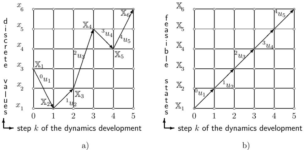
Fig. 2. The simplified representation of: a) the course of the DEDS state; b) the state trajectory in the state space
