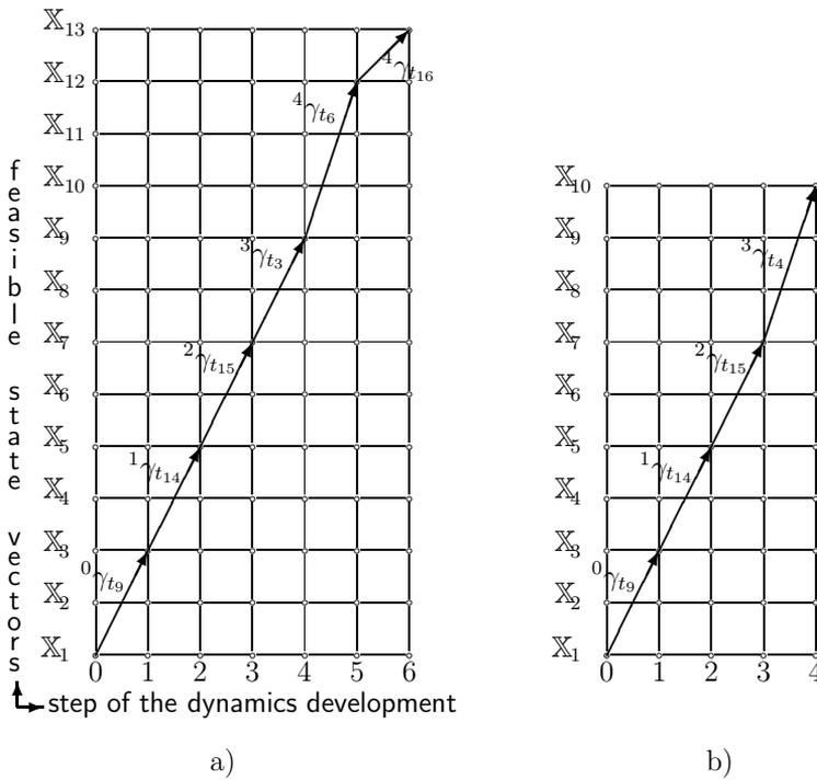
Fig. 11. The cooperation of two agents  $A1$ ,  $A2$  in MAS: a) the case when  $A1$  solves (on the basis of the demand of  $A2$ ) the problem to be solved by  $A2$ , however,  $A2$  is not able to do this; b) the case when  $A1$  refuses to help  $A2$
