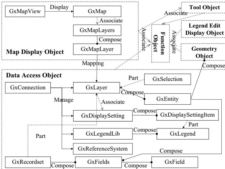
Fig. 5. Object diagram of the component layer
