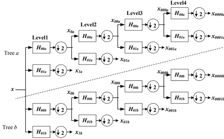
Fig. 1. The 1D Q-shift dual tree structure [21]
