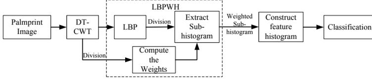
Fig. 5. The block of DT-CWT based LBPWH method
