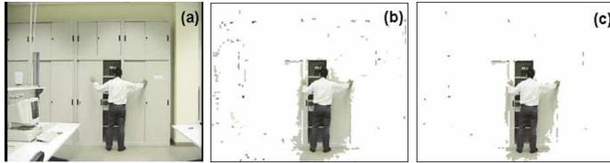
Fig. 8. Laboratory a) is frame 350; b), c) are detection results of HGMM without and with default minimum variance. (Default parameters:  $L = 30$ ,  $\alpha = 0.005$ ,  $T = 0.4$ ,  $T_h = T_m = 1$  s)
