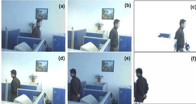
Fig. 9. Results of HGMM to handle sharp illumination changes without shadow elimination (Default parameters:  $L = 30$ ,  $\alpha = 0.005$ ,  $T = 0.4$ ,  $T_h = T_m = 2$  s)
