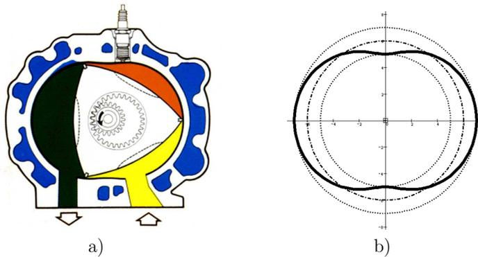
Fig. 6. The Wankel rotary engine
