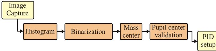
Figure 6. Processing stages of the eye tracking process
