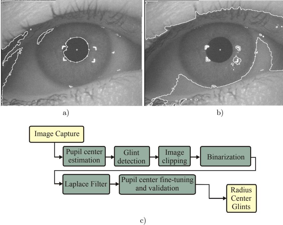
Figure 3. Processing stages associated to point of gaze detection: a) Determining pupil contour and center, b) Determining the radius of the iris, c) Summary of processing stages
