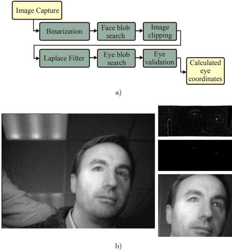
Figure 7. Face analysis for eye location: a) Eye location processing stages, b) Application example
