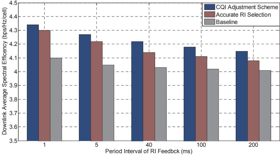
Figure 2. Downlink average spectral efficiency for InH scenarios
