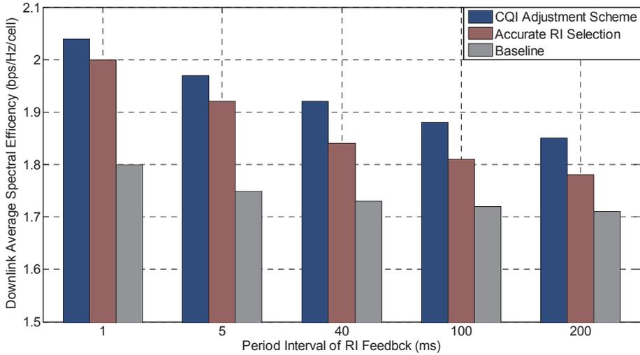
Figure 3. Downlink average spectral efficiency for RMa scenarios
