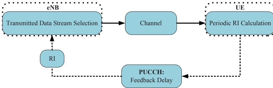
Figure 1. eNB and UE transmission principle of LTE systems
